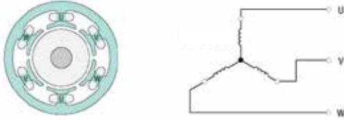
In the U, V, W line of the three-phase power supply, each phase is shifted by 120°. Since this phase shift creates a rotating magnetic field in the stator, it is unnecessary to connect a capacitor, such as with a single-phase motor.
