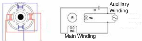
Connect the main winding to the power supply and the auxiliary winding to the power supply via the capacitor.
