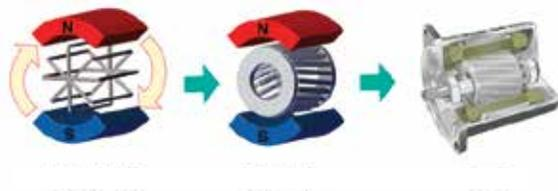
A squirrel cage rotor is a rotor with multiple skewed aluminum and iron bars. In a squirrel cage rotor, current flows in the aluminum part.
